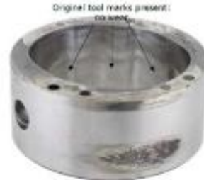
T6H20C Cam ring after 608h (with water)
