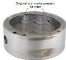
T6H20C Cam ring after 307h (no water)
