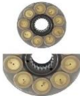
T6H20C Piston shoes after 307h (no water)
