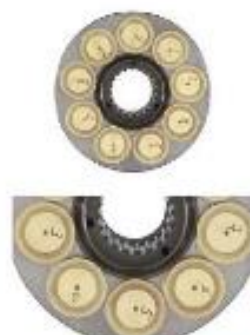
T6H20C Piston shoes after 608h (with water)
